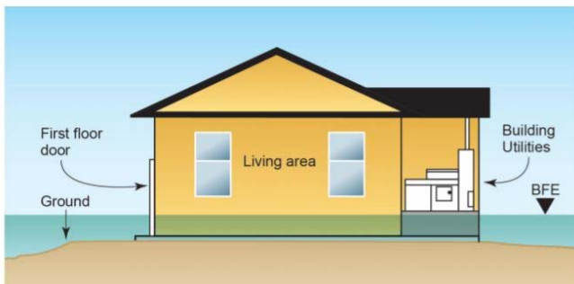
Figure 10: Elevation of building utilities (mechanical and electrical equipment) on platforms. (Source: FEMA P-1037)
