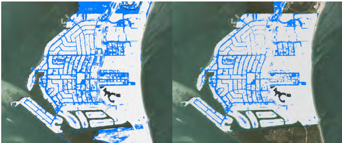
Fig. 8. The extent of tidal flooding (blue) in the Village of Key Biscayne projected to occur by 2045 under two scenarios: No Adaptation (left), With Backflow Valves (right). Note that the No Adaptation scenario (Figure 10, left) is identical to Figure 5 of Phase 1.
